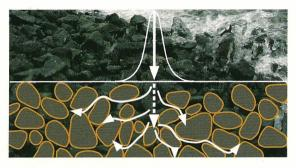
Elastocoast's chemistry creates a structure that offers both high porosity and high permeability; dissipating wave energy and reducing wave run-up for less coastline erosion.
